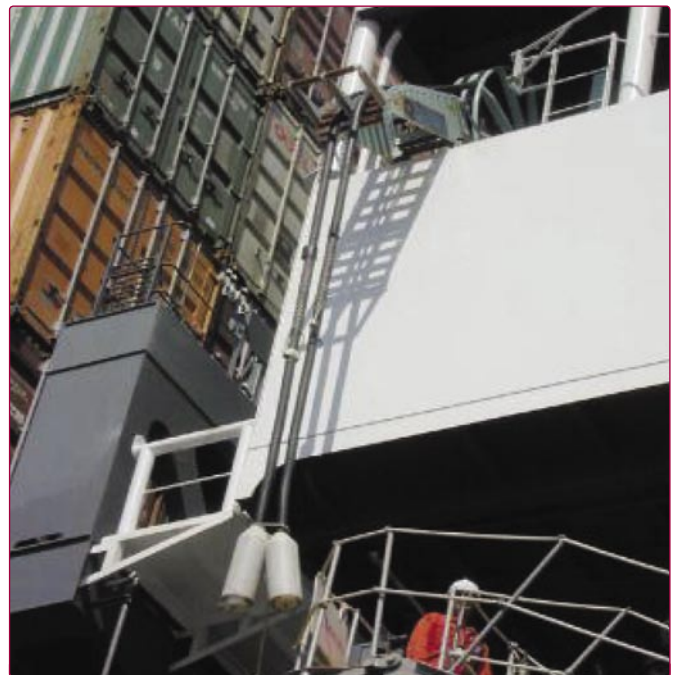
Figure 2. Plugs being deployed from ship.
