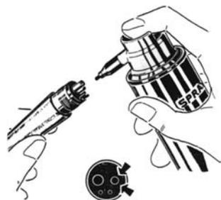
Fig. 10 - Lubrification piece a main
