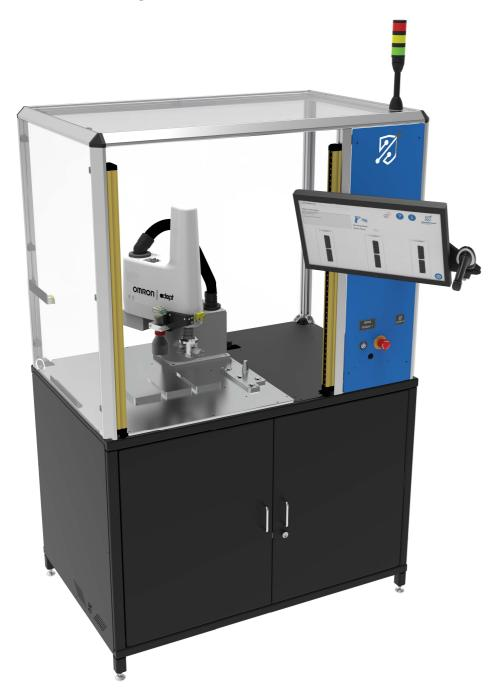
A robotic system designed to break plastic pins from connectors (punching system) in a fast and automatic way.
