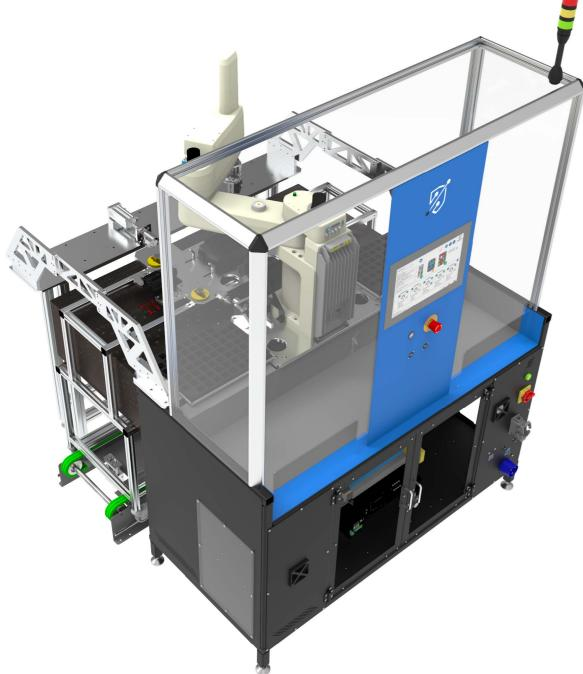
The AFRA - Relay Station, is a fully automatic system designed to insert relays into fuse boxes that are already mounted in the wire harnesses.
