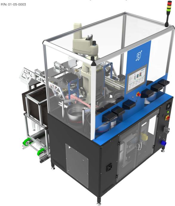
The AFRA - Fuse Station, is a fully automatic system designed to insert fuses into fuse boxes that are already mounted in the wire harnesses.
